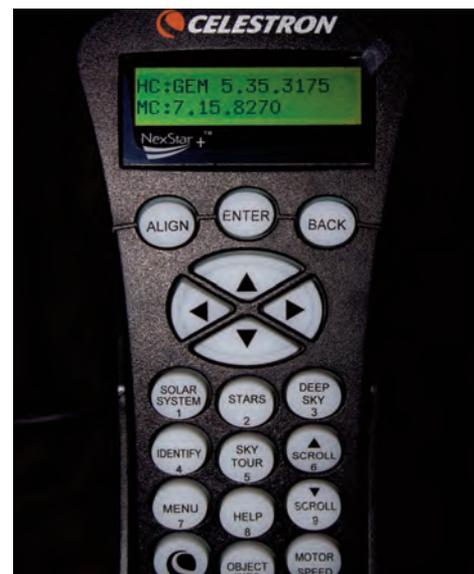
Image 15 – The hand controller must have firmware version 5.35 or newer to work with the StarSense Autoguider.
