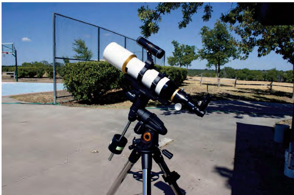
**Image 3** – The author attached the StarSense Autoguider to an Orion-style dovetail mount and attached it to the finder shoe on a small refractor.
