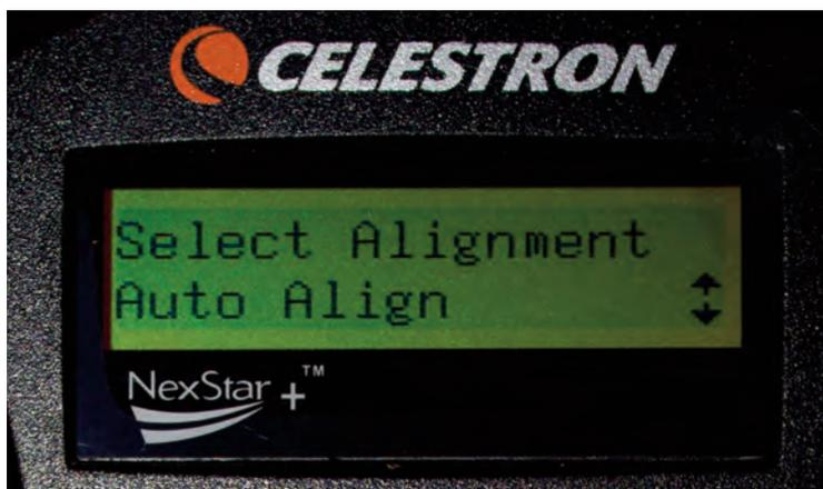
Image 17 – After skipping or completing a polar alignment with the StarSense Autoguider, the next step is to use it to star align the mount.
