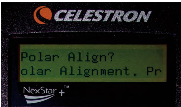
Image 16 – With the StarSense Autoguider attached to the telescope, the first operation it tries to perform is a polar alignment of the mount.
