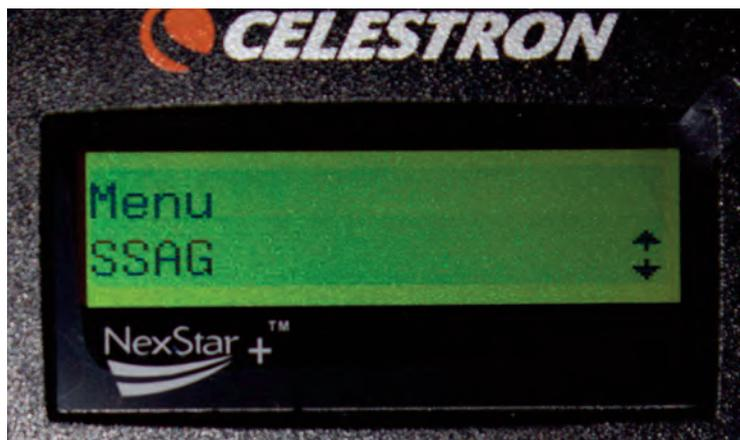
Image 19 – The SSAG menu is used to access features of the StarSense Autoguider.
