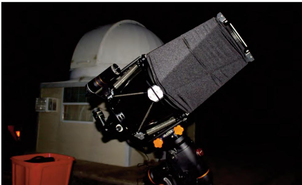
Image 14 – Another view of the StarSense Autoguider, 10-inch Cassegrain telescope, and CGEM-DX mount.
