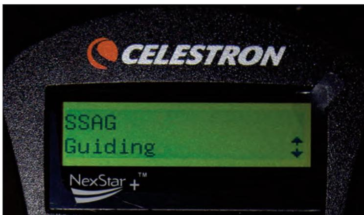
Image 22 – To initiate guiding from the hand controller, use the guiding menu found under the SSAG menu.
