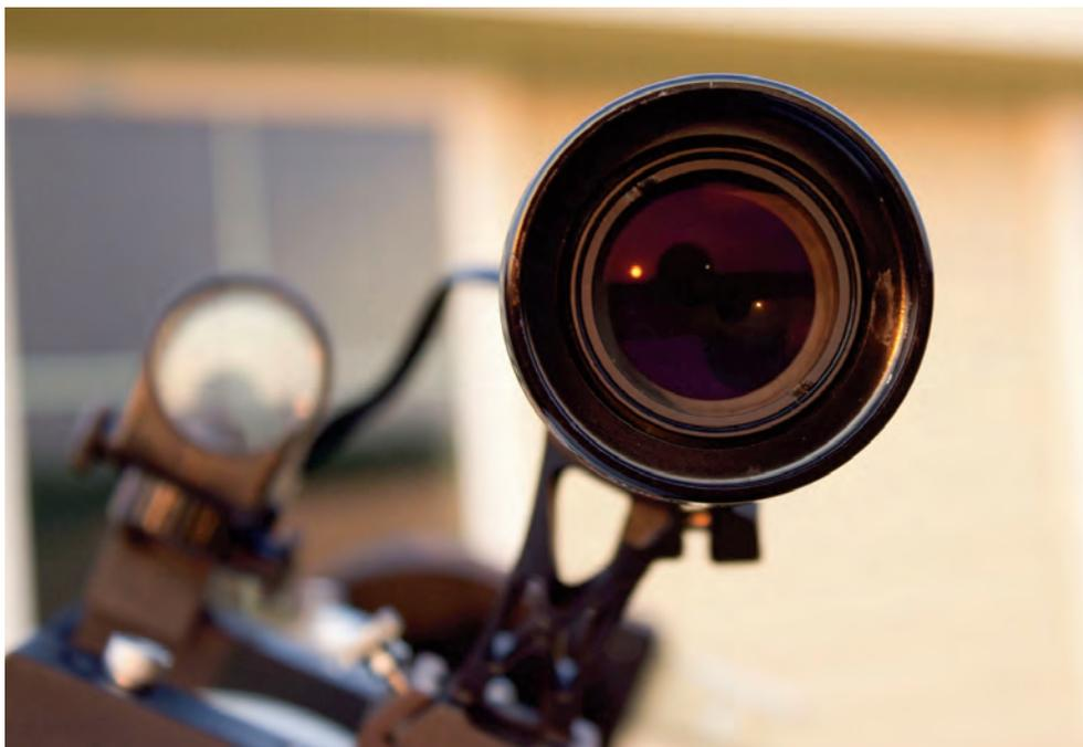
**Image 6** – This view shows the StarSense Autoguider's optics.
