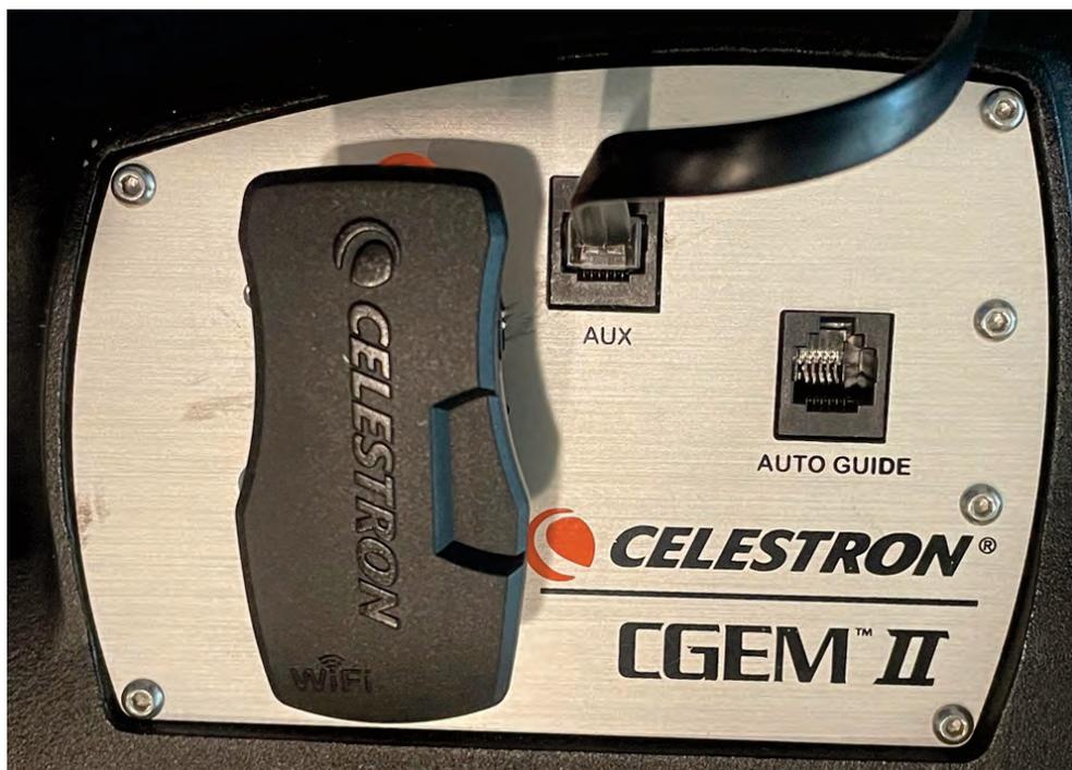
**Image 8 – The StarSense Autoguider’s auxiliary cable should be attached to the AUX port on a Celestron mount. It can be controlled via a phone, tablet or computer using WiFi from a Celestron SkyPortal adapter shown here**
