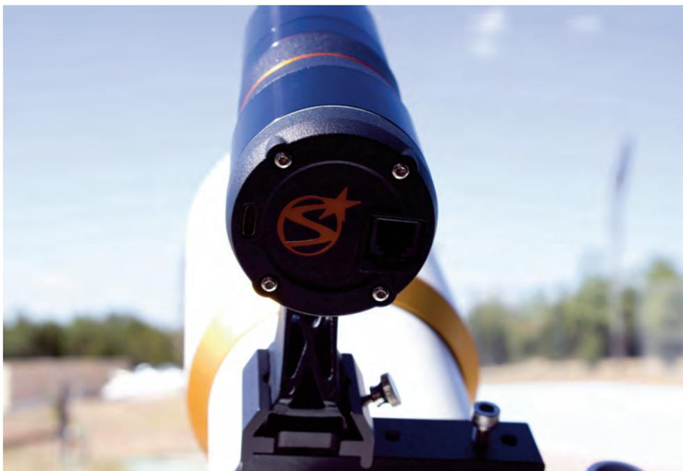
Image 5 – The back of the StarSense Autoguider has two ports. One for connecting an auxiliary cable to the mount and one for connecting a USB cable to a computer to upgrade its firmware
