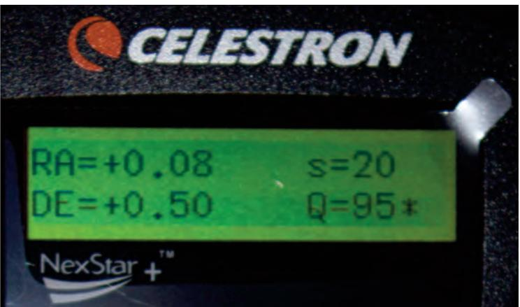
Image 23 – Guiding RMS errors are displayed for both axes. The "s" number indicates 20 stars are used for guiding. The "Q" number rates the atmospheric seeing.
