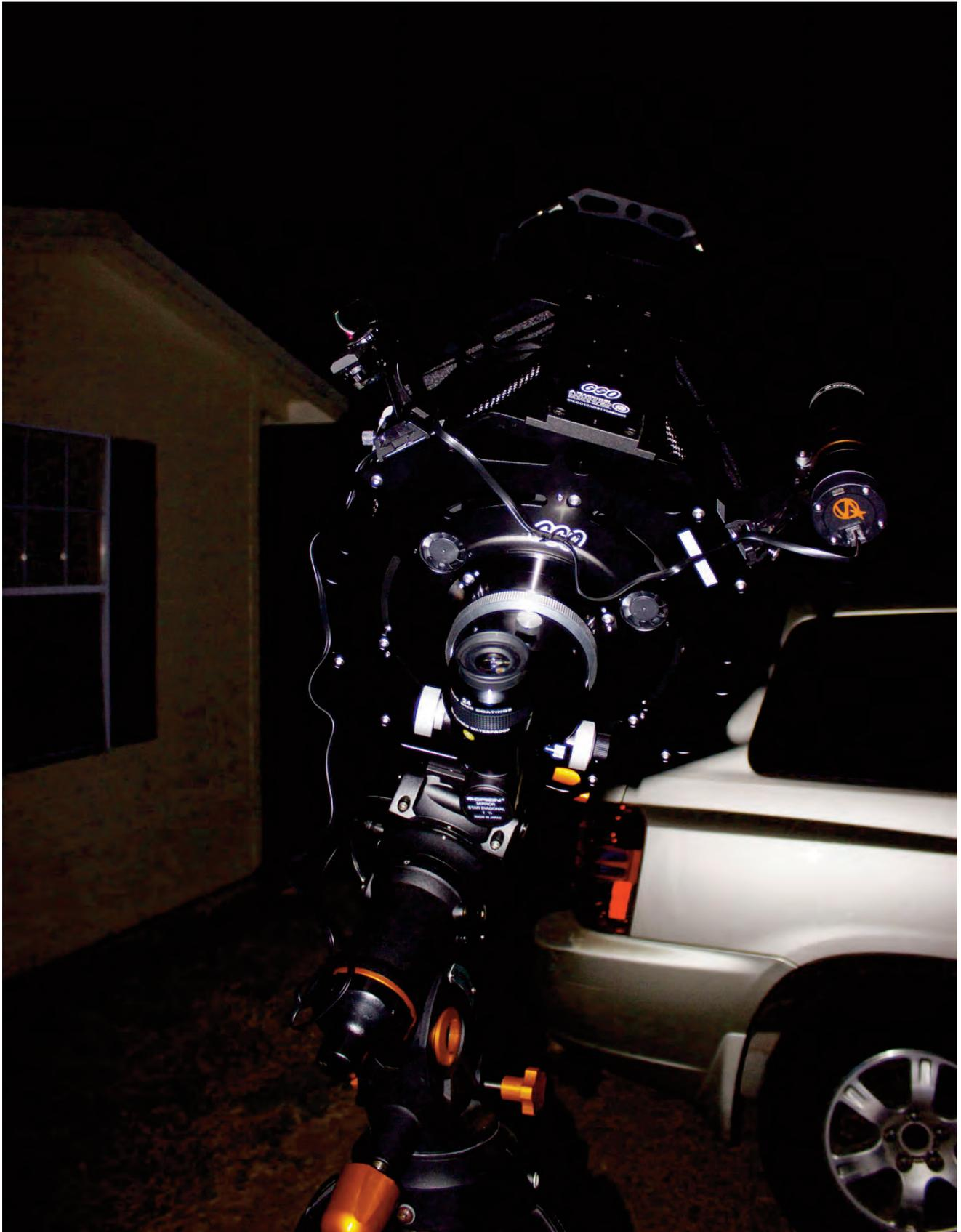
**Image 12 – The author attached the StarSense Autoguider to a 10-inch f/12 classical Cassegrain on a Celestron CGEM-DX mount to test the GOTO capabilities with a long focal length instrument.ware.**
